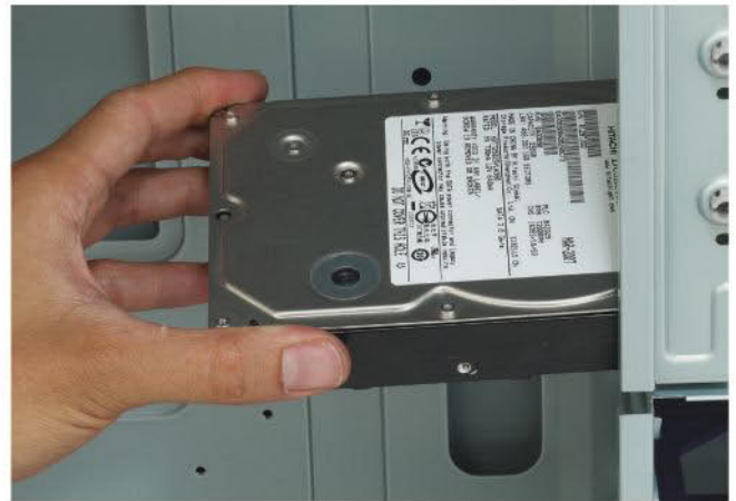
▲ Create a NAS from an old PC by filling it with spare hard disks
